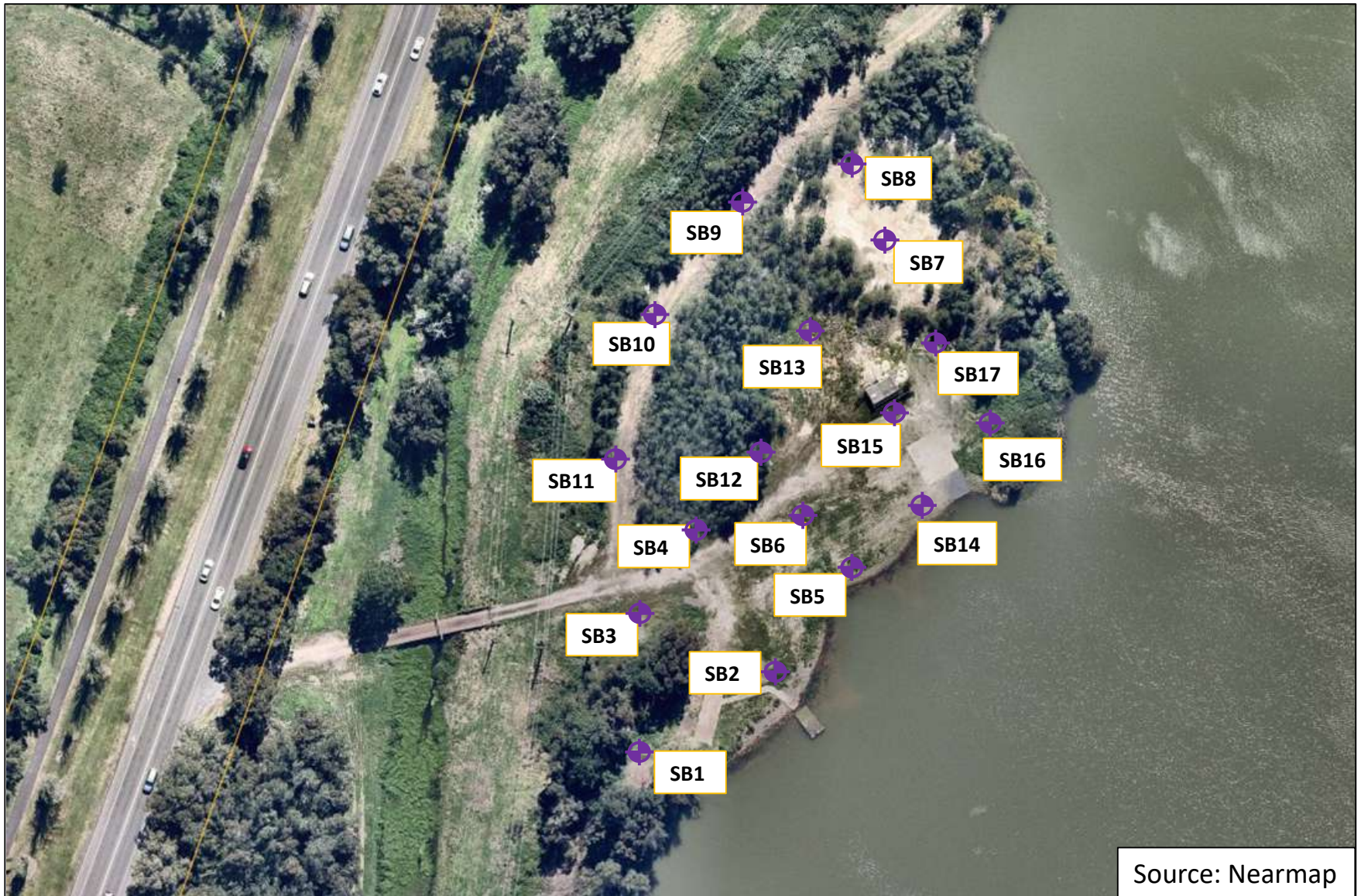
Figure 1: Indicative Contaminated Land Assessment Area and GW Monitoring Well Location Plan
